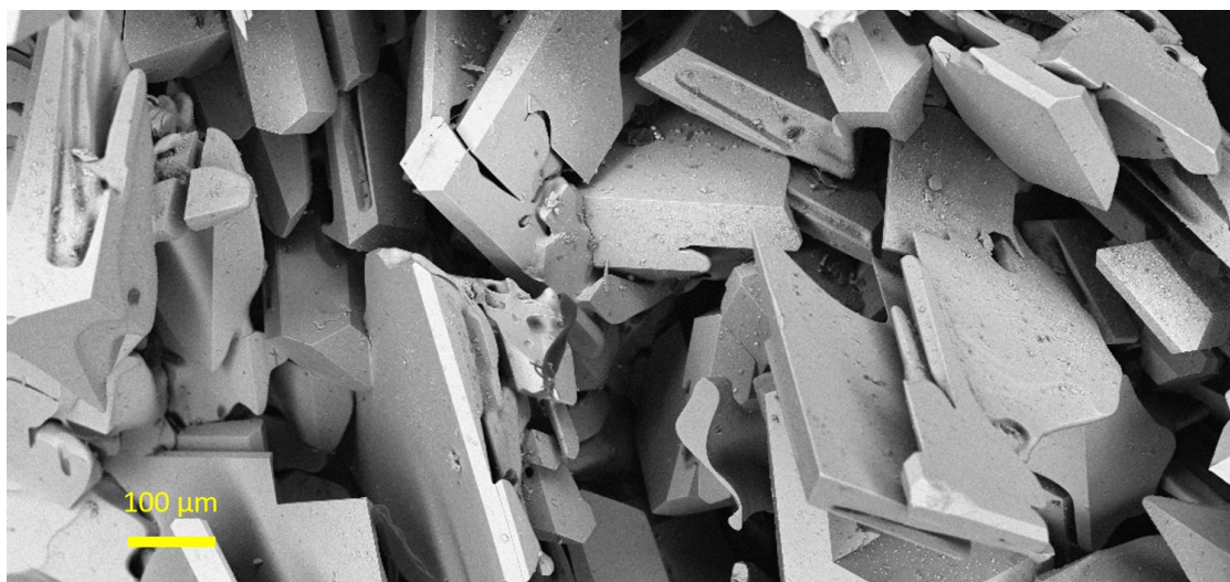
SEM image of an aggregate of iron chalcogenides crystals grown in a molten chloride flux.
