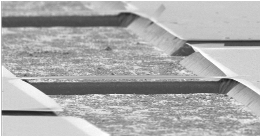
Scanning electron microscope micrograph and optical picture of a strained 150×15 μm 2 microbridge fabricated from a 100 nm thick LSMO single crystalline film
